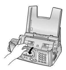
3 Clean the document feeder rollers (①) and rubber flap (②) with a cloth moistened with isopropyl rubbing alcohol, and let all parts
